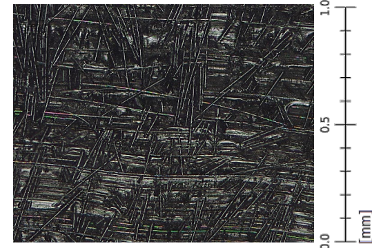
Surface far away from injection point adhesive fracture between tape and thermoplast
