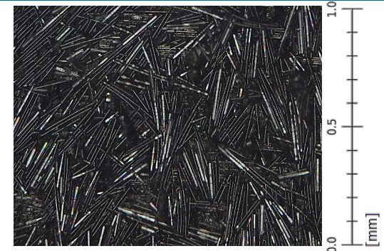
Surface next to injection point cohesive fracture in thermoplast
