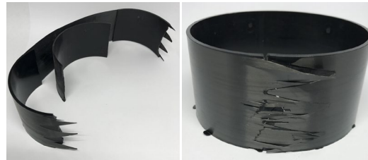
Delamination vs. fiber fracture
