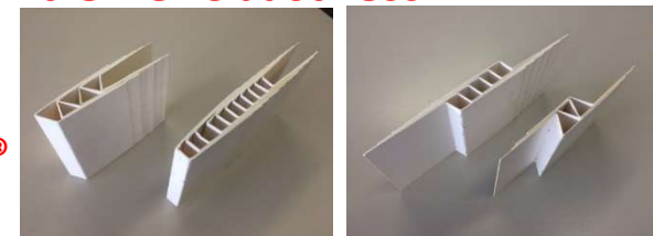
Multiple impact damage + fatigue = local delamination, no damage growth
