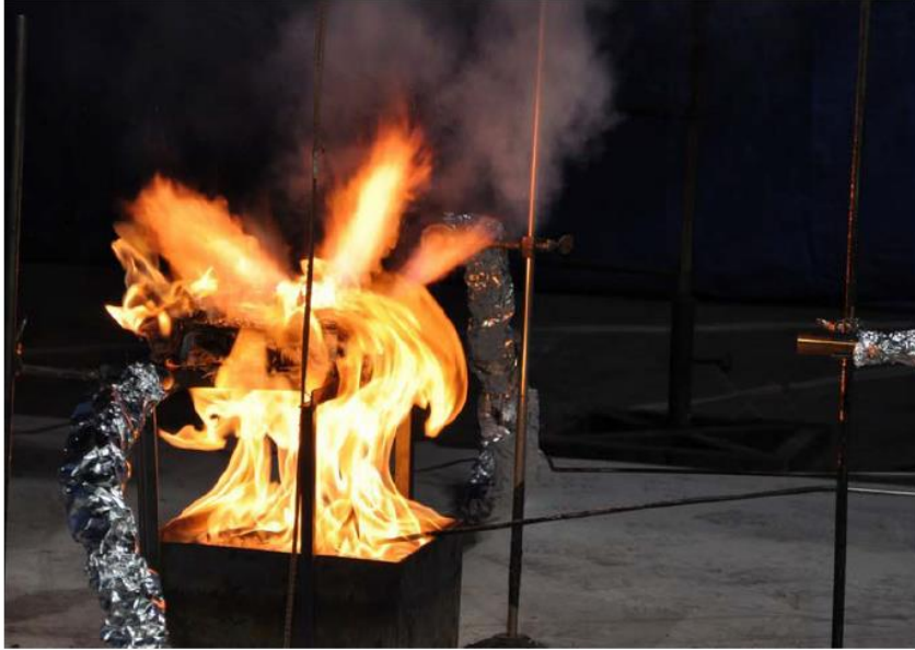
Photo 3- Venting of the electrolyte from a battery exposed to fire. General Civil Aviation Authority of the UAE
