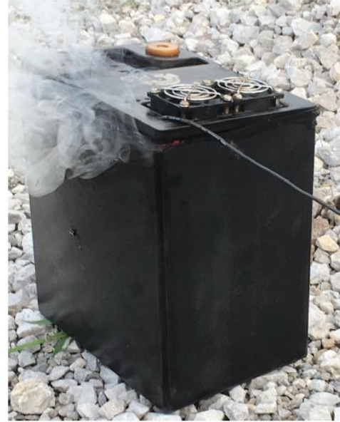
Battery box containing Li-ion cells, manufactured with PS200 prepreg, after a full thermal runaway 15-minute test. Internal temperature 1100°C, external face temperature 200°C. Photo courtesy of SHD Composite Materials Ltd.
