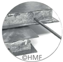
Aluminum foam sandwich with integrated steel tubing
