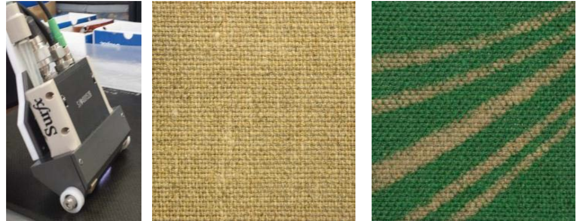
Plasma source, flax fibres before (left) and after selective treatment
