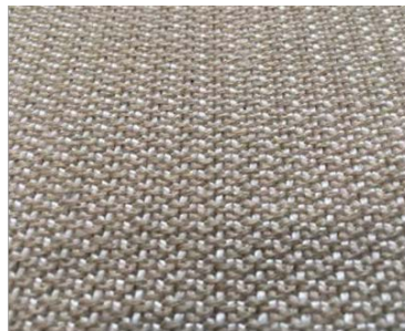
hybrid woven fabric, flax and thermoplastic matrix
