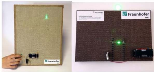
Flax multi-layer hybrid fabric with PA6 and integrated LED
