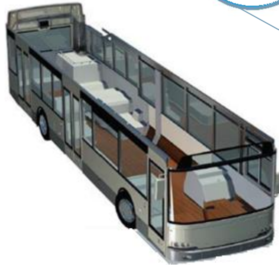
Pre-assembled sandwich module directly bonded on bus/coach walls
