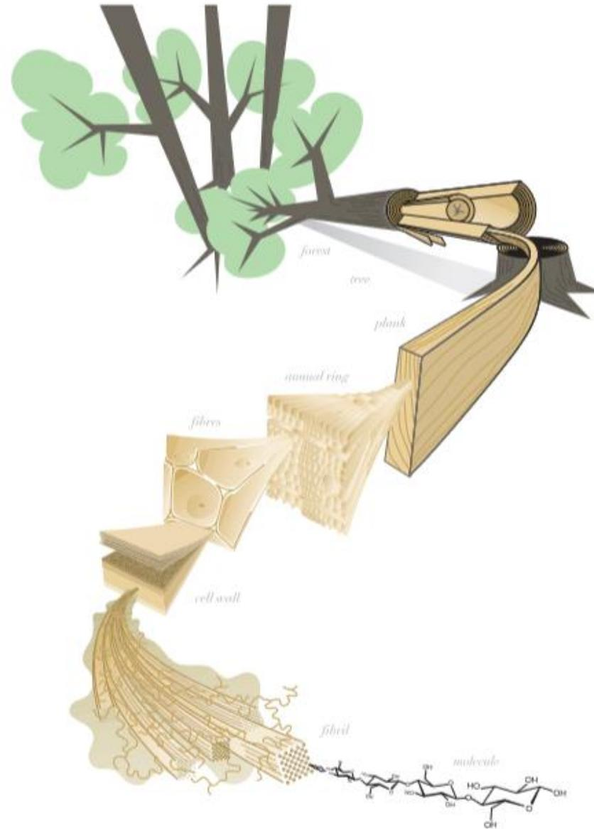
Figure 3. Hierarchical structure from the tree to the molecular level (Illustration: Airi Illiste).
